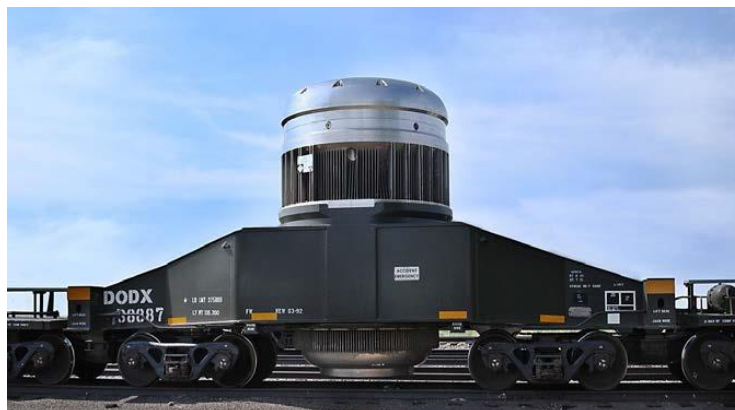
Figure 7-2. Railroad Shipping Container used by the U.S. Navy to Transport High-Level Waste
