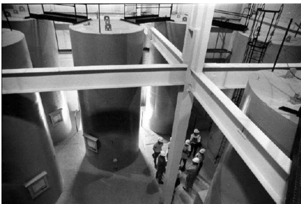
Figure 5-1 Spent Fuel Casks at Gentilly-1
