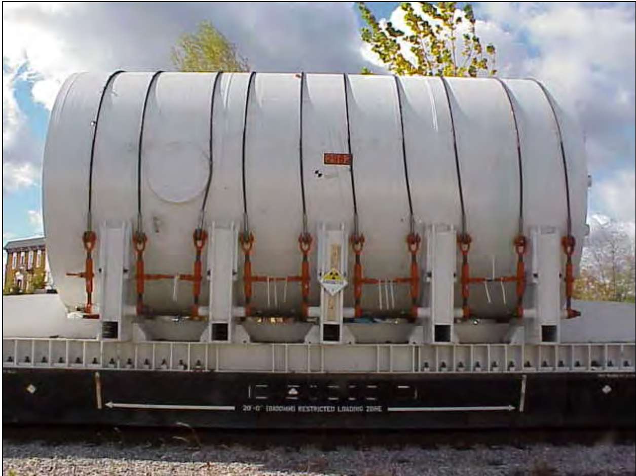
The reactor vessel packaged for shipment by rail for disposal at the EnergySolutions low-level radioactive waste disposal site in Barnwell, South Carolina.
