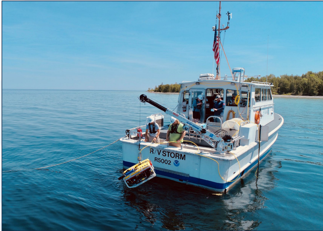
NOAA GLERL engineers deploying a remotely operated vehicle to install flow meters in Lake Huron, July 2019 Credit: David J Ruck, Great Lakes Outreach Media
