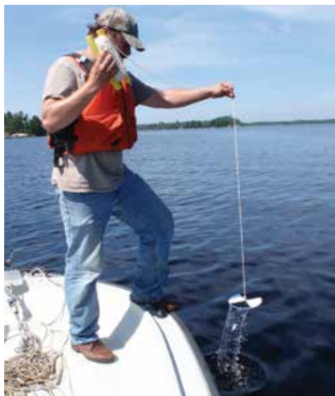
Measuring water quality with a Secchi disk. (U.S. NPS Staff Photo)
