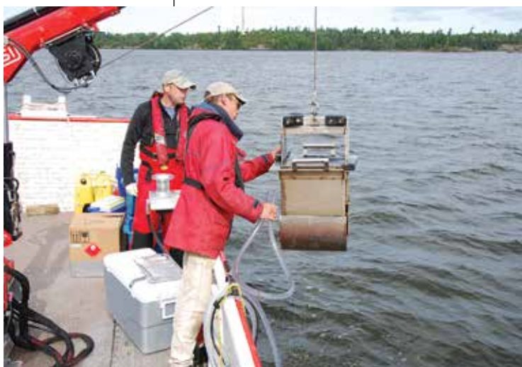
Sediment sampling by Environment Canada (Environment Canada)
