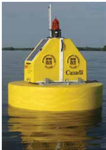
Water quality monitoring buoy. (Environment Canada)
