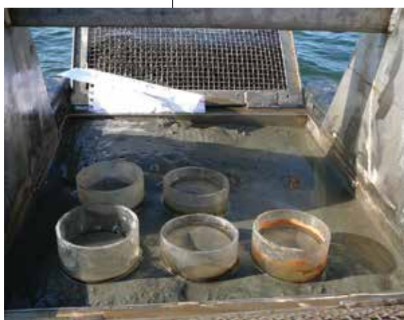
Sediment subsampling by Environment Canada (Environment Canada).
