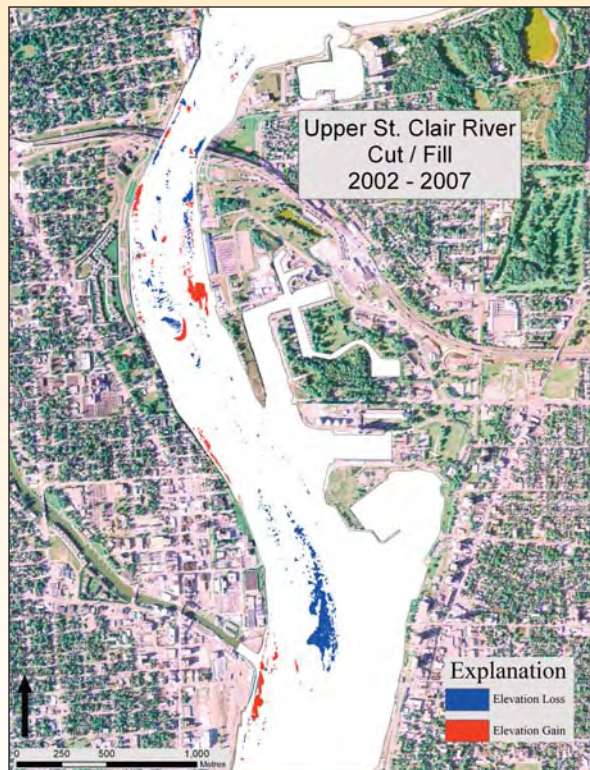
Figure 4-7 Detectable Net Bed Elevation Changes in the Upper St. Clair River from Multi-Beam Swath Surveys (2002-2007)
