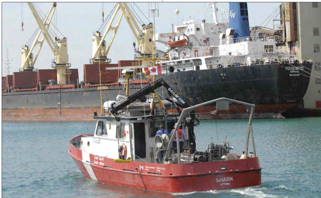
Researchers used the Department of Fisheries and Ocean's Shark to carry out bathymetric surveys on the St. Clair River. Such surveys need to be conducted on a regular basis to help improve understanding of how the river bed reacts to changing conditions.
