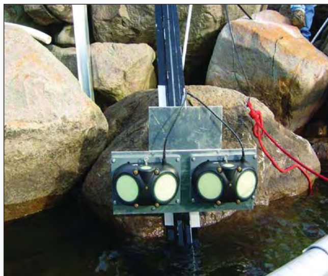
A new hydrometric (water quantity) gauging station on the St. Marys River, one of four new stations on the connecting channels of the upper Great Lakes installed under the Study. Government support for the continued operation of these stations after the Study is completed will provide key data to help Canada and the United States manage the Great Lakes under a changing climate regime.
