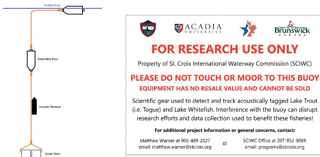
Figure 9 Diagram (left) portraying the layout of each of the acoustic receiver moorings deployed across East Grand Lake, ME/NB, in addition to the signage (right) placed on each of the subsurface & surface buoys to deter public interaction with the equipment.
