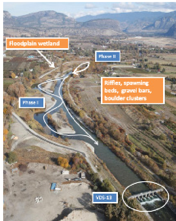
Figure 8. ORRI Phase I, II and VDS 13. Restoration of oxbows, a side channel and parts of an historic floodplain. Source: Okanagan Nation Alliance.
